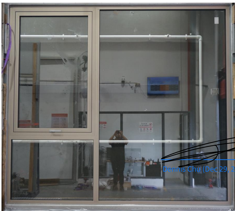
Figure 2 Photo of the test specimen Before testing (Fully Closed)
