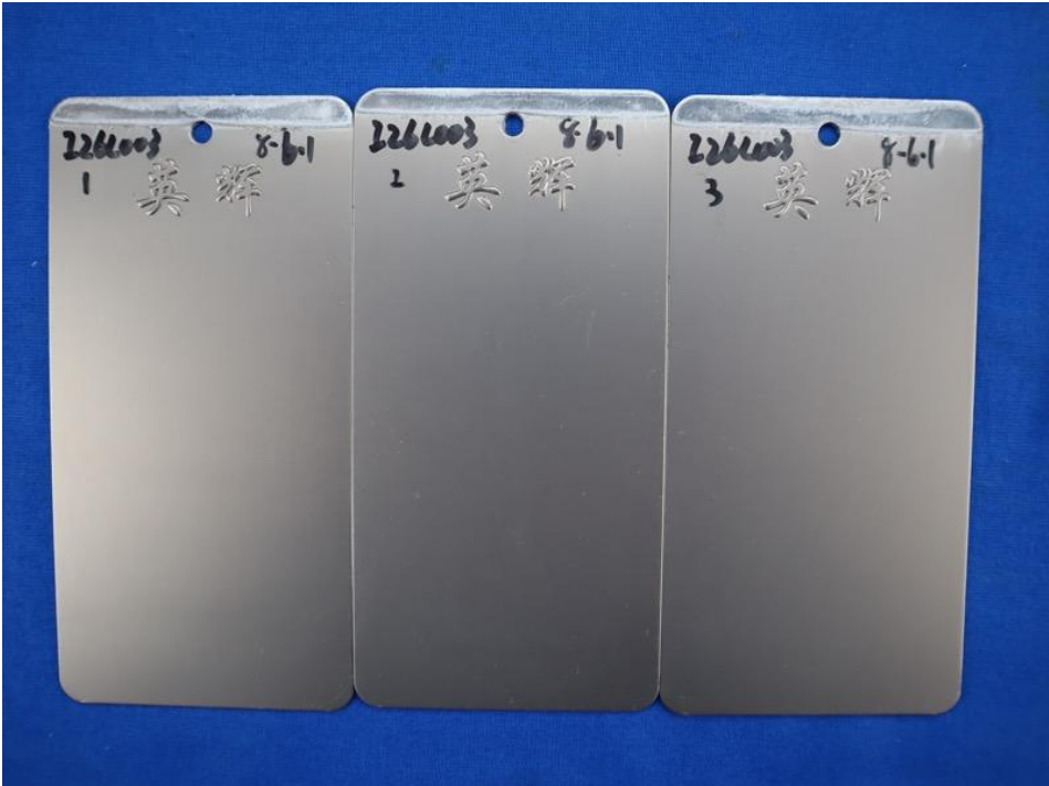
Figure 5 – Samples after Muriatic Acid Resistance test (see Ch. 2.6.1: Test acc. to AAMA 2603-22, Ch. 8.6.1)
