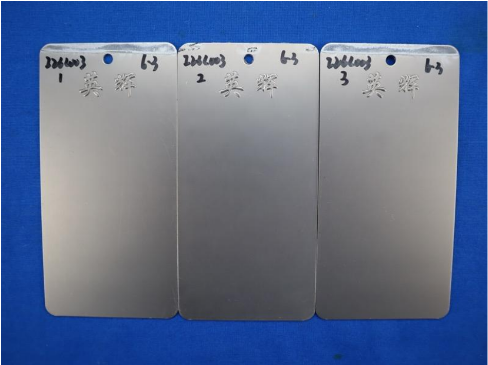
Figure 7 – Samples after Detergent Resistance test (see Ch. 2.6.3: Test acc. to AAMA 2603-22, Ch. 8.6.3)
