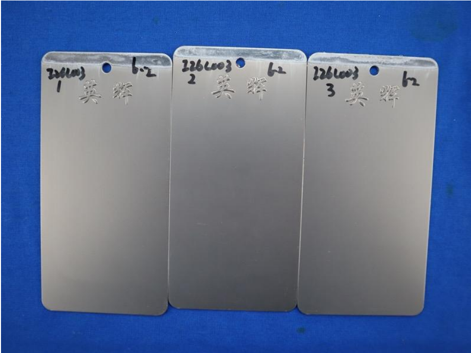
Figure 6 – Samples after Mortar Resistance test (see Ch. 2.6.2: Test acc. To AAMA 2603-22, Ch. 8.6.2)
