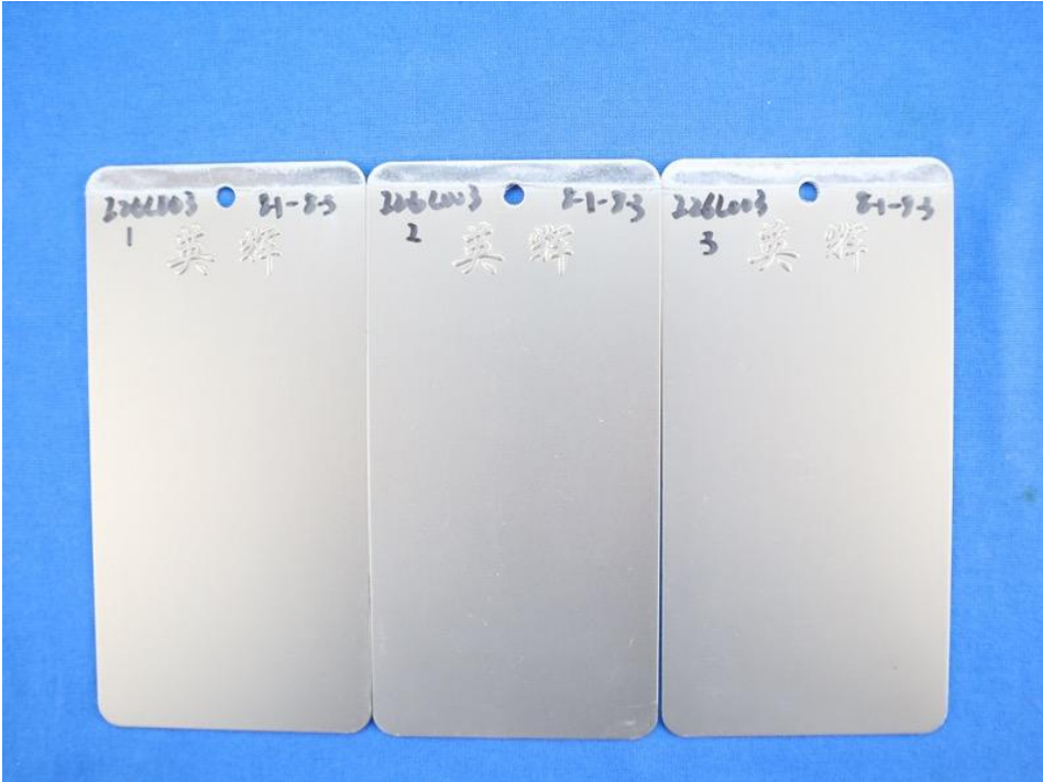
Figure 2 – Samples for Color Uniformity and Specular Gloss and Dry Film Hardness test (see Ch. 2.1 and 2.2: Tests acc. to AAMA 2603-22, Ch. 8.1&8.2&8.3)
